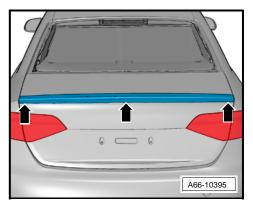
Check the lateral adhesive joint -Arrows- and adjust the position of the spoiler of necessary.
